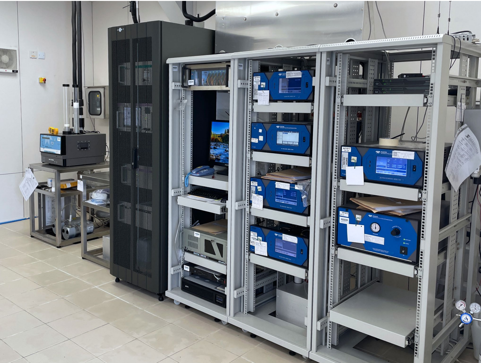
Figure A2: Instrument for measuring the air pollutants at an AQMS.
